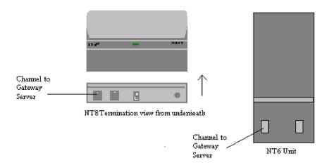
The gateway system connects to the ISDN  ${\tt 2}$  using a pre-installed UTP cable . The cable is terminated at each end with an RJ45 male connector.
