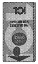
You must insert the card into the smart card reader on the keyboard, with the front of the card facing you and the broad arrow pointing downwards.
